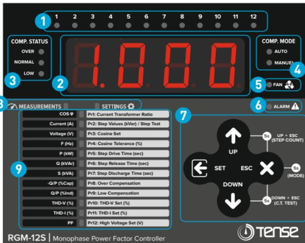
**1- Step LEDs:** These are the LEDs that light up when the steps are active.
